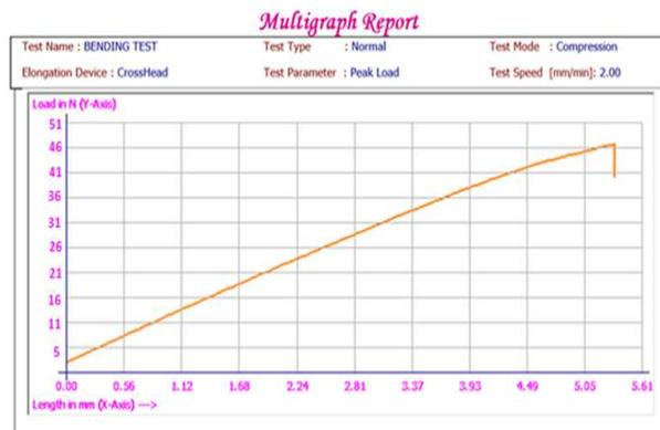
**Figure 8: Multi Graph Report for Flexural Test 5 % Weight Fraction.**
