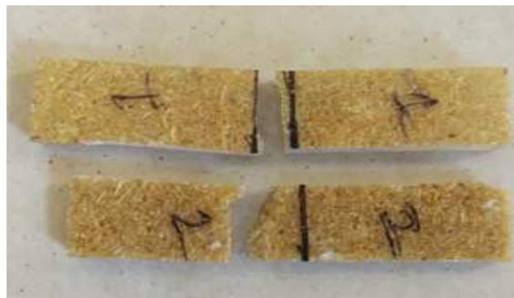
**Figure 7: Tested Specimens after Impact Test.**
