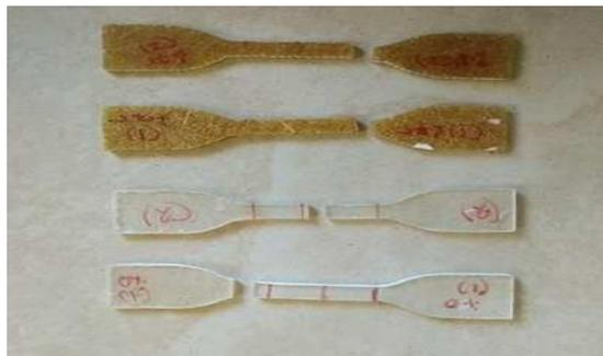
**Figure 5: Tested Specimens**
