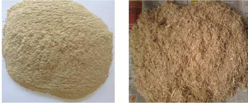
**Figure 1: Sugarcane Bagasse Fibre.**
